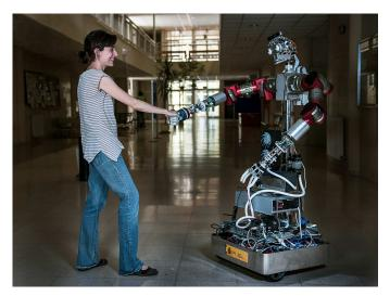
Fig. 1: The mobile manipulator Loki
