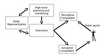
Fig. 3: Outline of the RoboCog architecture.
