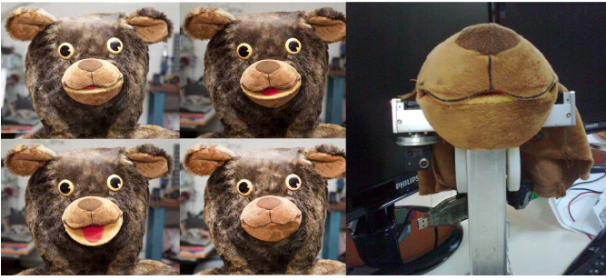
Fig. 4. In the left hand side it can be seen the robotic mouth mounted on the Ursus 2 robot. In the right hand side it can be seen the mouth system separated from the rest of the robot, as used in section VI.
